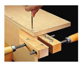
However, a straight-shanked screw isn't a cure-all. Even when using a pilot hole and the right screw, MDF can still split out. So one final precaution is to support the sides by clamping an ordinary hand screw across the work piece, see the photo at left. It makes it almost impossible to split the MDF.
